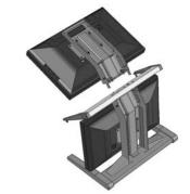
4. Thread the cables from the top monitor through the rectangular hole in the cross bracket.
